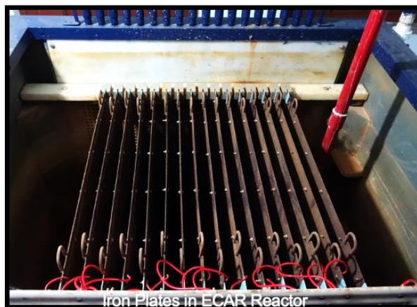
Iron Plates in ECAR Reactor
